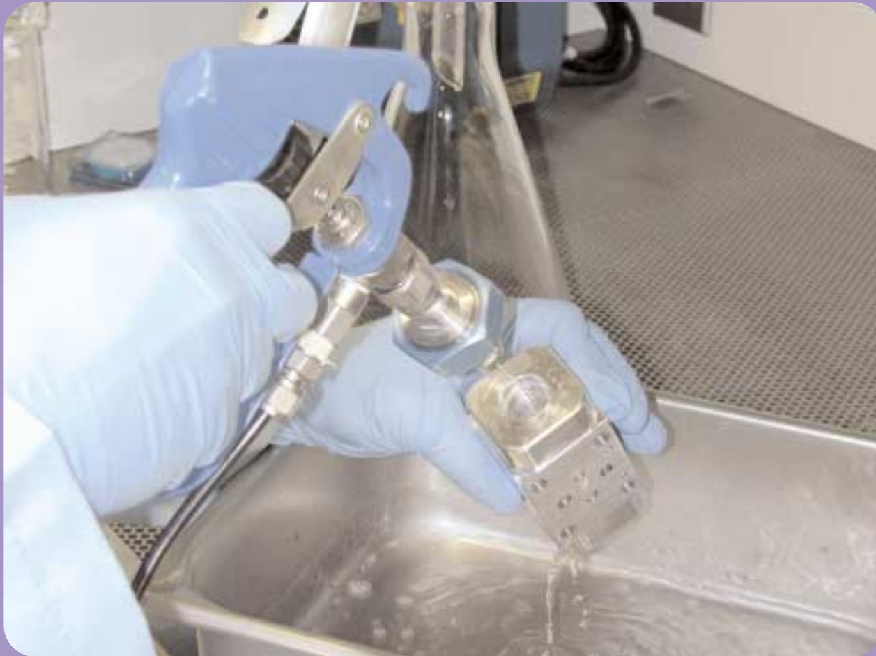
Solvent Rinsing of Washed Parts
