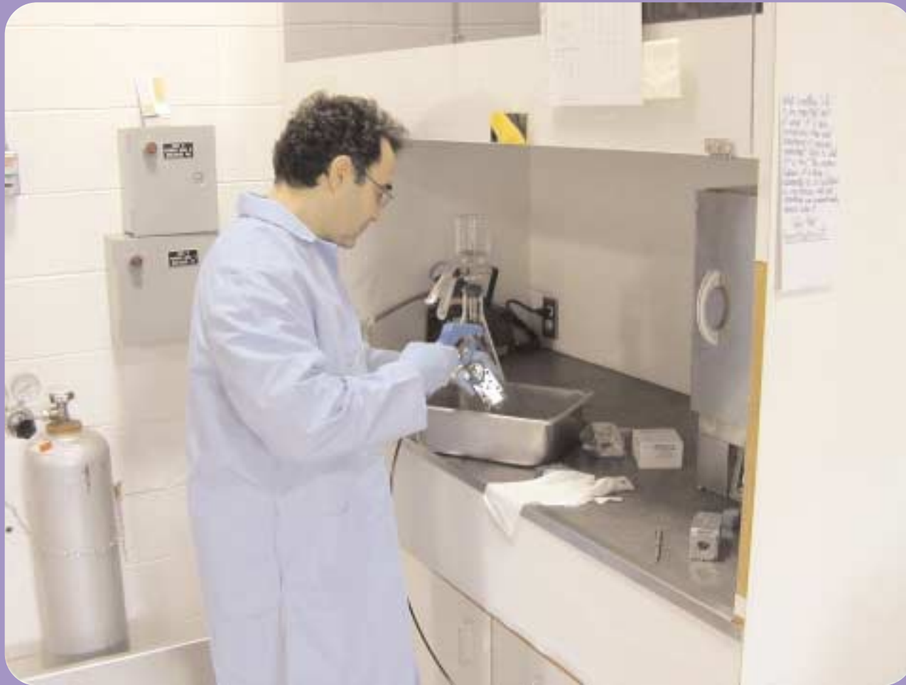
Solvent Rinsing of Washed Parts
