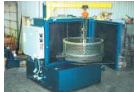
48" Turntable w/Overhead Hoist
